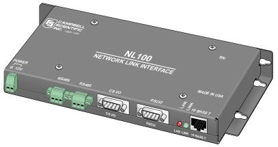
Communication from the base station computer is supported by PC208W (Version 3.2 or higher) for our array-based dataloggers, LoggerNet for our table-based dataloggers, and PC9000 for the CR5000 and CR9000(C) dataloggers. Communication rate is dependent on the datalogger; for example, the CR5000 can communicate at rates up to 115,200 bps.
